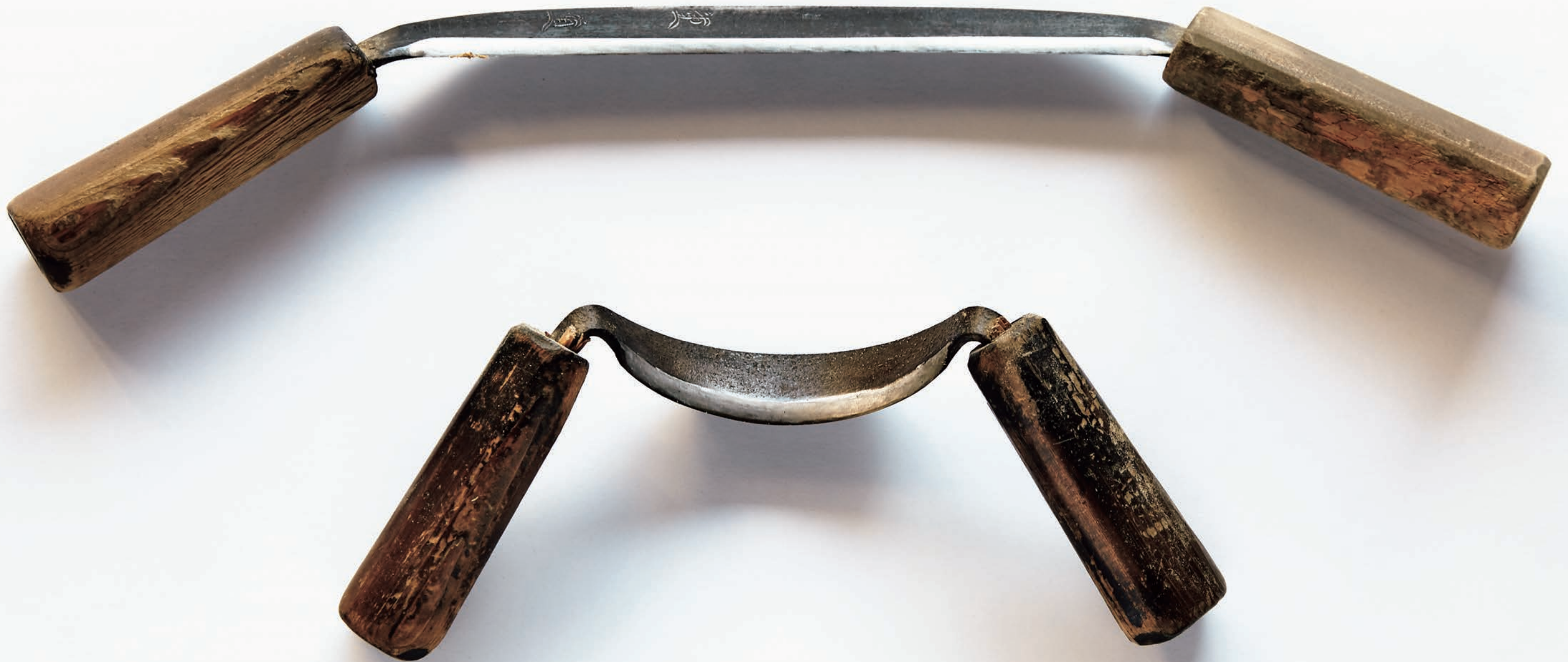
A sen is a plane with a handle on each end used to shave side slats. Sen come in a variety of sizes and shapes to accommodate slats of varying size and curvature. In the past, there were even artisans who specialized in making tools for making oke .
